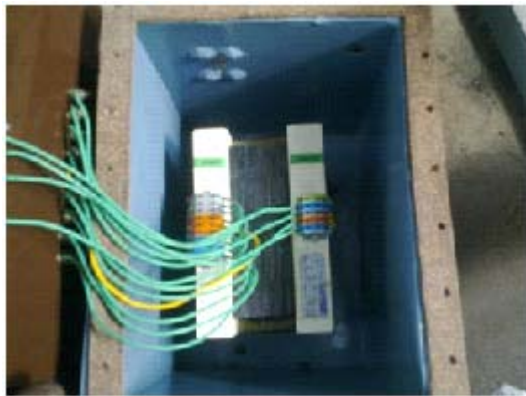
Fig. 9. Windings of 1KVA Prototype Transformer
