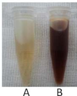
Fig. 1. Color changing of the aqueous extract of Ziziphus vulgaris after formation of the SNPs. A: blank and B: extract containing SNPs.
