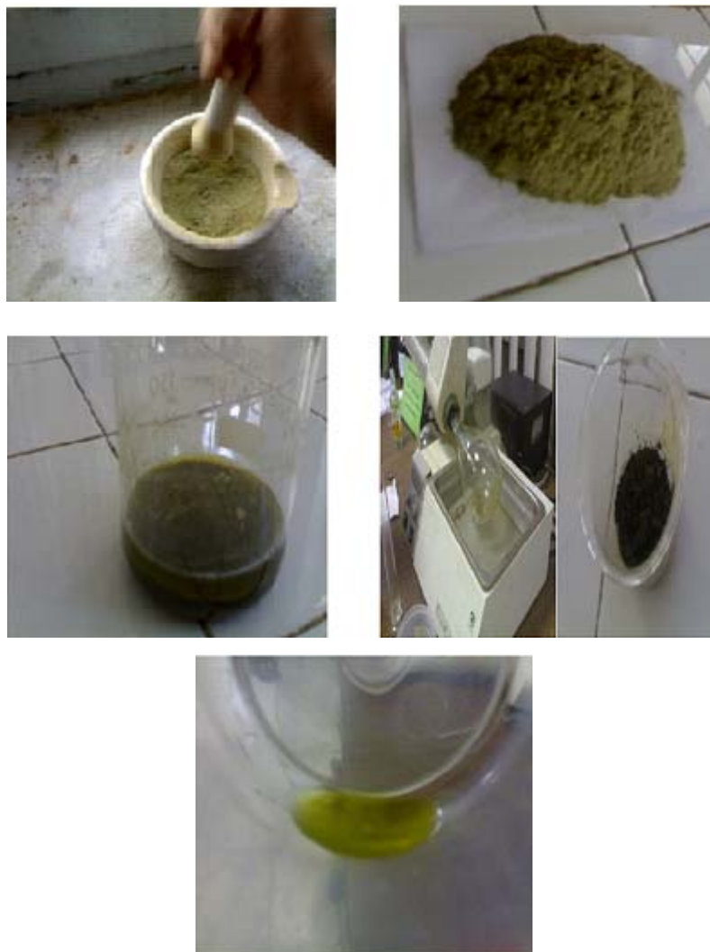
Fig. 2. Stepwise process of extraction (a) grinding of algae (b) grounded algae (c) mixing of solvents and biomass (d) evaporation of solvent in rotary evaporator (d) extracted oil
