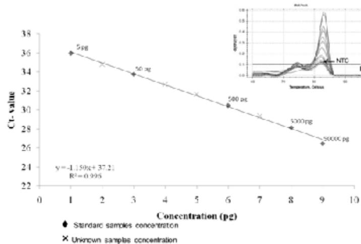
**Fig. 10 a.** Standard curve obtained with marker BKF2 and BKR2 by correlation of cycle threshold number ( $C_T$ ) value to the log of *R. solani* DNA concentrations. **b.** Dissociation curve analysis of amplicons produced by *R. solani* specific marker BKF2 and BKR2 with template DNA and non-template control.
