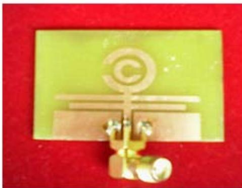
Fig. 12. Fabricated CDSRR antenna with stub
