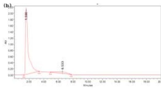
**Fig. 5.** (a) HPLC chromatogram of biodegradation of monocrotophos in soil with nutrients; (b) HPLC chromatogram of biodegradation of monocrotophos in soil without nutrients.
