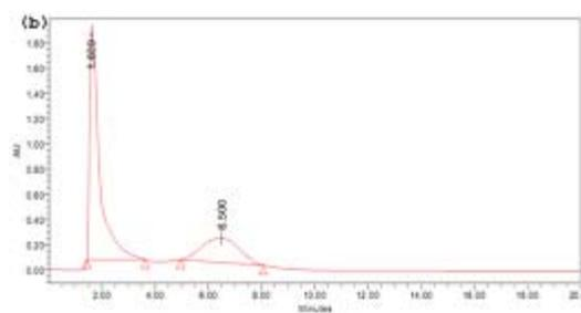
**Fig. 4.** (a) The HPLC chromatogram of monocrotophos at standard condition (b) HPLC chromatogram of biodegradation of monocrotophos in aqueous medium by *Aspergillus oryzae* SJA1.
