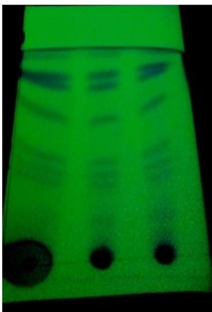
**Figure 4.** TLC to analyze the band separation in the solvent system of chloroform: methanol (ratio of 9:1, 8:2 and 7:3).
