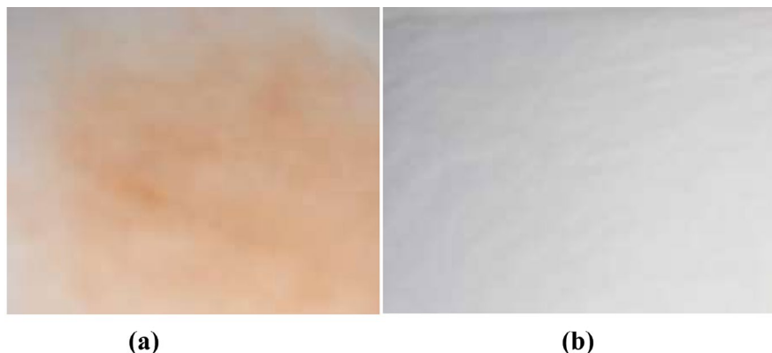
Fig. 7. Images of anti-redeposition effect of mannanase with tennis court clay on cotton cloth (a) without mannanase (b) with mannanase.
