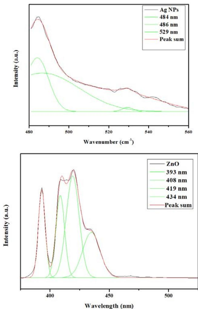
**Fig. 4.** Photoluminescence spectrum of Ag and ZnO NPs.
