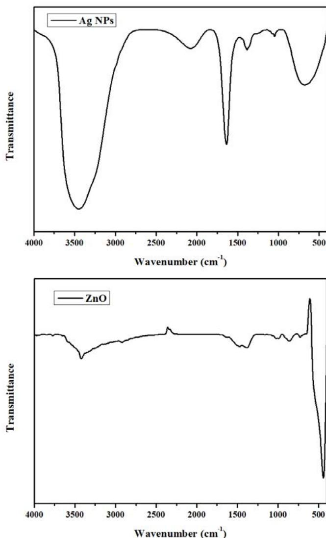
**Fig. 3.** FTIR spectra of Ag and ZnO NPs
