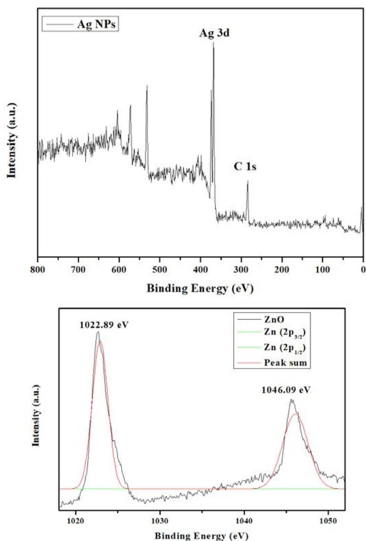
**Fig. 2.** XPS wide spectra of Ag and ZnO NPs green synthesized by leaf extracts
