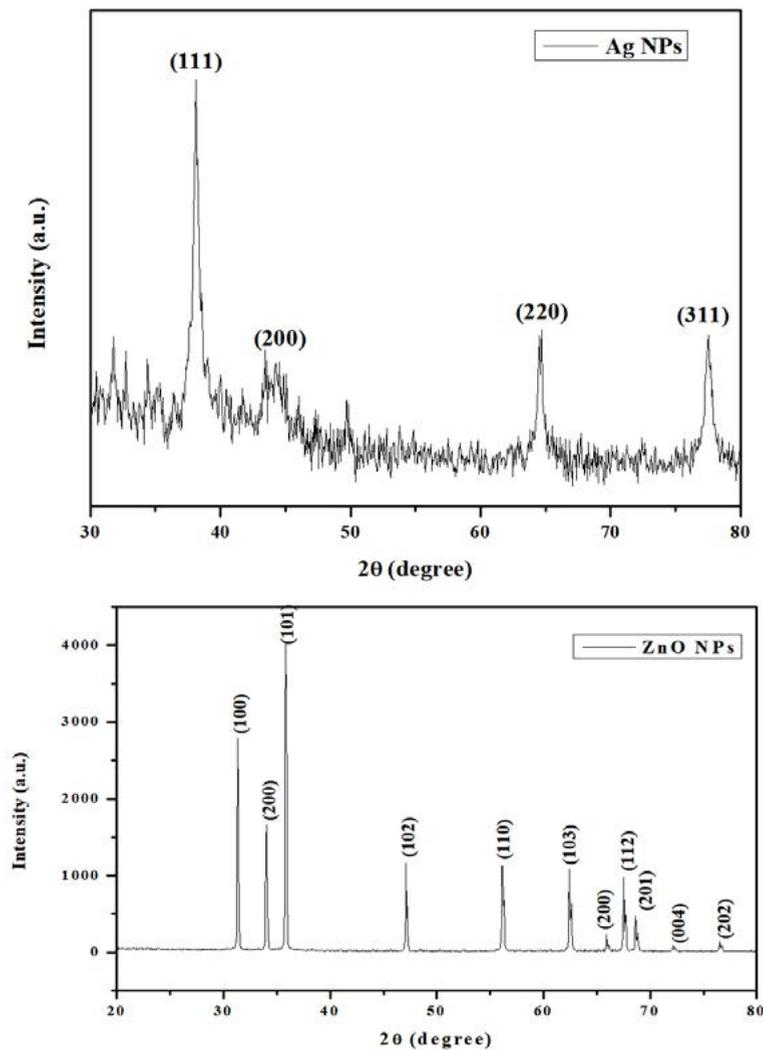
**Fig. 1.** XRD patterns of green synthesized Ag and ZnO NPs using *Phyllanthus niruri* and *Aristolochia indica* leaf extracts
