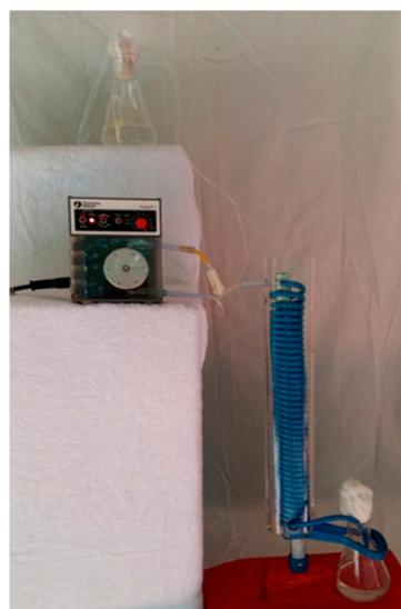
Fig. 1. Working condition of PU based bioreactor
