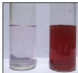
Fig.1. Biosynthesis of silver nano particle by green synthesis (a) initial inoculum of the extract with silver nitrate precursor. (b) Silver nano particle biosynthesis after 30 minutes of incubation
