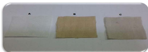
Fig. 9. Removal of tea stains by crude tannase from A. nomius GWA5. (A) control; (B) Piece of cotton cloth treated with tap water; (C) Piece of cotton cloth treated with crude tannase.
