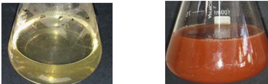
a) MRS broth culture with 10ml of selenium-based solution includes, (NaHSeO3), and inoculated strains of L. acidophilus and L. plantarum is equal to half McFarland before incubation b) Selenium nanoparticles production and color change after 48-72 hours incubation at 37 °C medium with 50rpm in MRS broth culture.
