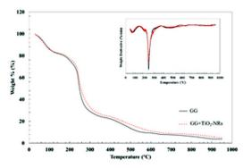
Fig. 5. TGA thermogram of GG and GG+TiO<sub>2</sub>-NRs films
