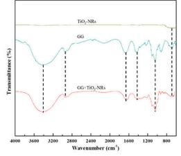
Fig. 3. FTIR spectra of  $\text{TiO}_2$ -NRs, GG, and GG+TiO $_2$ -NRs films
