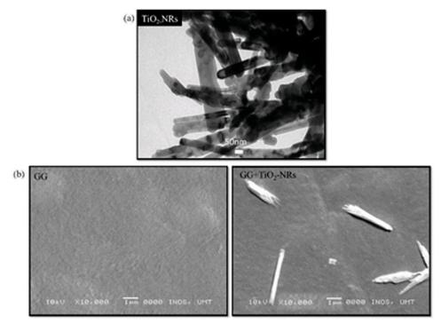
Fig. 2. (a) TEM micrographs of TiO<sub>2</sub>-NRs (b) SEM micrographs of GG and GG+TiO<sub>2</sub>-NRs films
