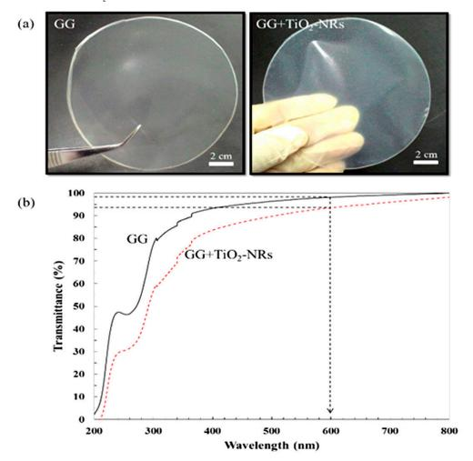
Fig. 1. (a) Physical appearance of GG and GG+TiO,-NRs (b) UV-Vis transmittance of GG and GG+TiO,-NRs films
