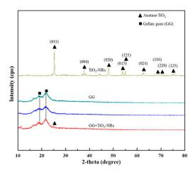
**Fig. 4.** XRD diffractogram of TiO<sub>2</sub>-NRs, GG, and GG+TiO<sub>2</sub>-NRs films
