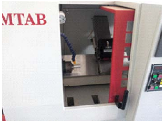
Fig. 1. Application of cutting fluid during an experiment
