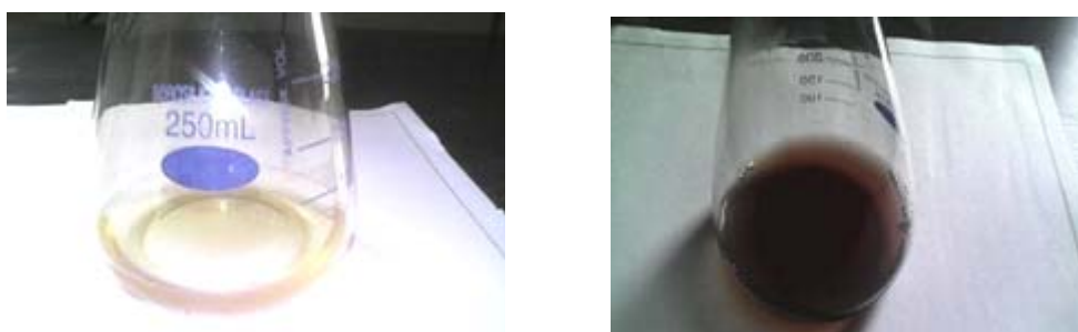
Fig. 1. Synthesis of silver nanoparticles (AgNPs) using G. lucidum extract. (a) G. lucidum mycelial polysaccharide extract. (b) Polysaccharide extract treated with AgNO 3
