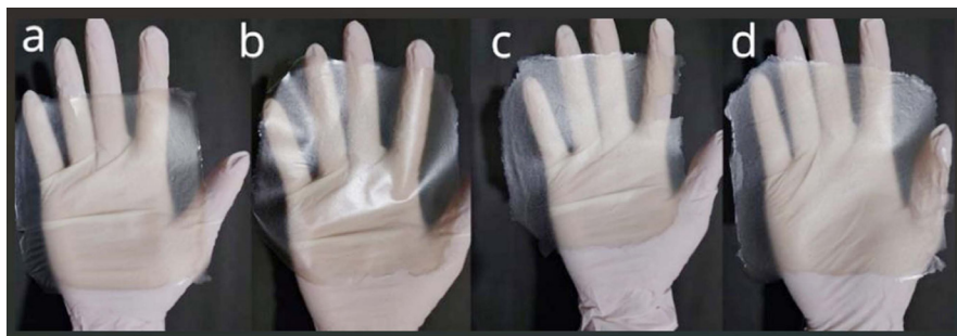
Figure. Appearance of dry casein-konjac edible film incorporating basil leaf extract: (a) Control (0% extract) (b) 5% extract (c) 6% extract (d) 7% extract
