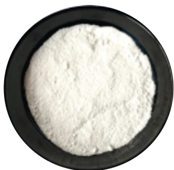
Figure 3. The above image depicts the freeze dried formulation of microbes. This is referred to as freeze dried cell powder biofertilizer formulation which is created by cultivating beneficial microorganisms, harvesting their biomass, and subsequently freeze-drying (lyophilizing) the material. This procedure maintains cell viability, stability, and shelf life by removing water under low temperature and vacuum
