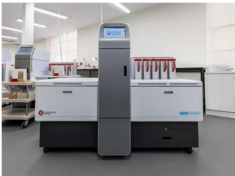
Figure 6. The APAS Independence: Intelligent imaging and machine learning technology to read and interpret the presence of significant bacteria in culture plates. (Source: https://cleverculturesystems.com/technology/intelligent-automation/apas-independence )
