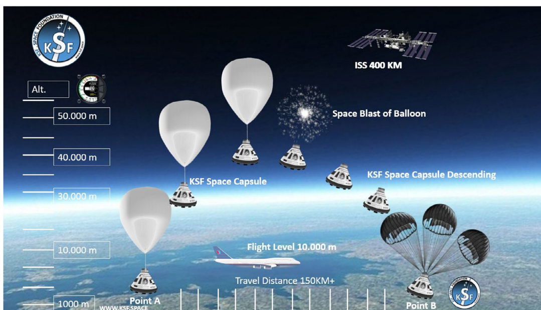
Figure 1. A BalloonSat simple package designed by the KSF Space Foundation was used to carry out lightweight experiments in near space. The design is under weight and volume constraints, which allows for the inclusion of several BalloonSat during flight. The airframe material is lightweight Styrofoam or foam core, which provides reasonably good insulation (Source: KSF Space, Nevada, United States)
